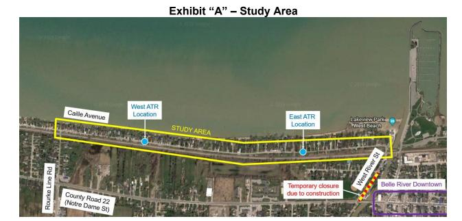
It should be noted that the current pavement width on Caille Ave. is approximately 6m, which is less than ideal. A typical width would be 8.5m for an urban residential local road. Further, the roadway has numerous driveways and mature trees along it which is a hindrance to drivers. These road characteristics alone would be cause for lower operating speeds.
