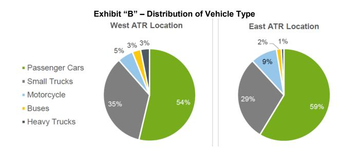
Post-construction, daily traffic volumes were observed to be in the 700-950 vehicles per day range. Overall, measured speeds were higher for passenger cars and small trucks in the range of approximately 53 km/h on average which certainly exceeds the 40km/h current posted speed limit. These speeds may pose some risk to the residents and pedestrians in the area. There was a significant change in traffic patterns following construction.
